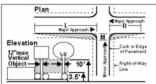
In Sight Triangle: Only vertical objects 12" or less in diameter, from 3.5 to 10 feet above street grade.
