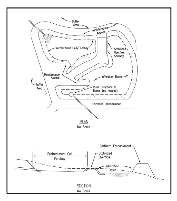
FIGURE 14.01-1 Infiltration Basin – Plan and Section
