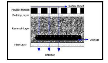
Figure 14.04-1. Cross Section of Typical Permeable Pavement (Source: Hunt & Collins, 2008)
