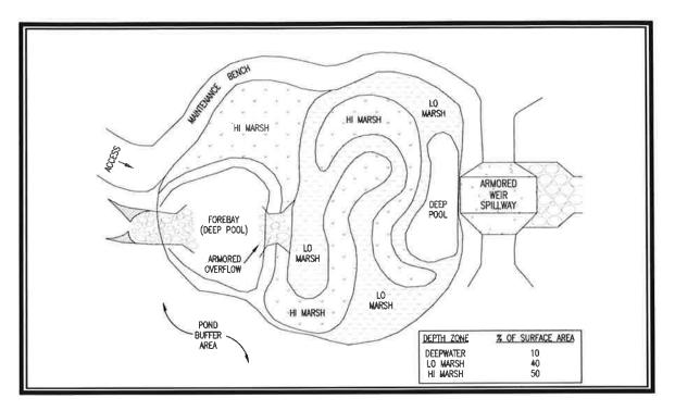
FIGURE 14.05 - 1 Constructed Stormwater Wetlands - Plan
