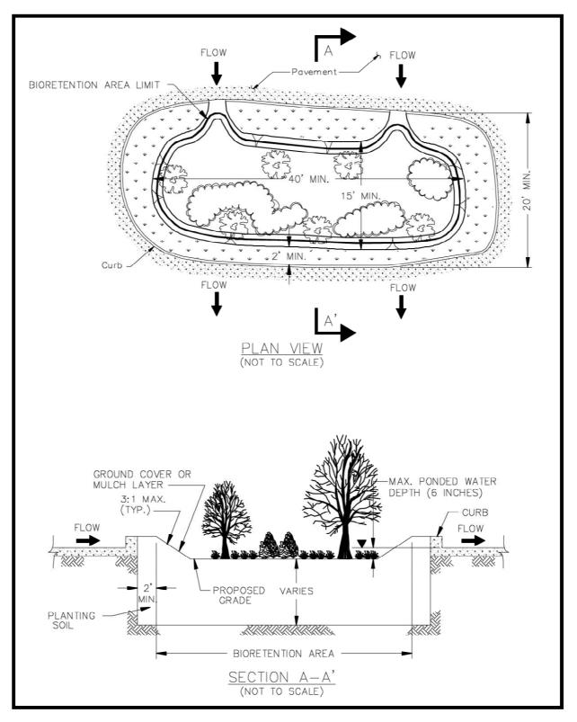
FIGURE 14.08-3 Bioretention Basin in a Planting Island in a Parking Lot
