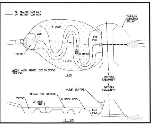
FIGURE 14.05- 3 Dry Weather and Wet Weather Flow Paths
