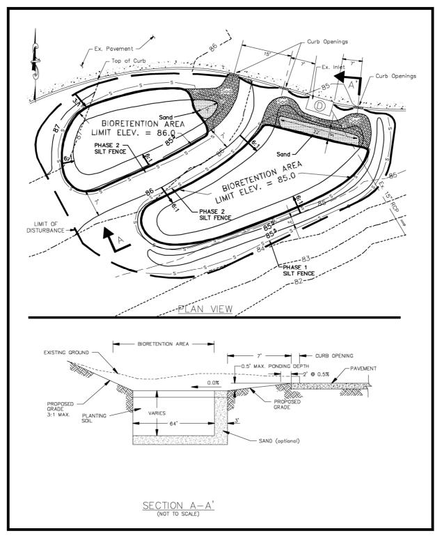
FIGURE 14.08 – 7 Grading Plan for Bioretention Basin
