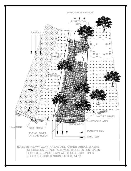
FIGURE 14.08-1 Bioretention Basin
