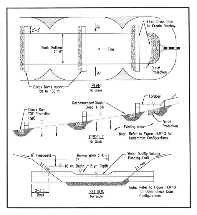
FIGURE 14.07-1 Typical Grassed Swale Configuration
