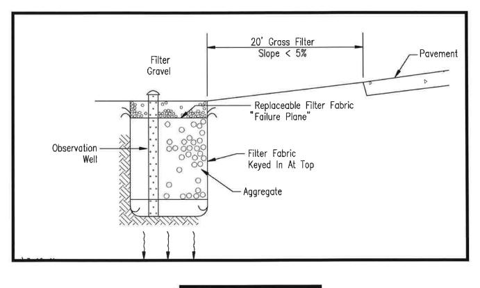
FIGURE 14.02-1 Infiltration Trench - Section
