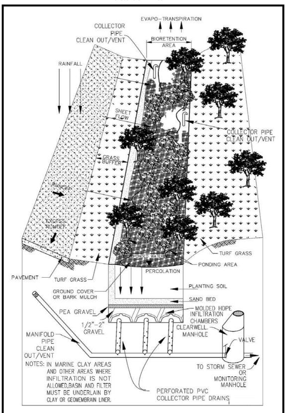
FIGURE 14.09A-1 Bioretention Filter
