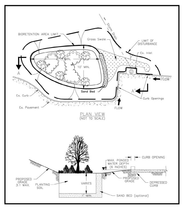
FIGURE 14.08-2 Bioretention Basin at Edge of Parking Lot With Curb
