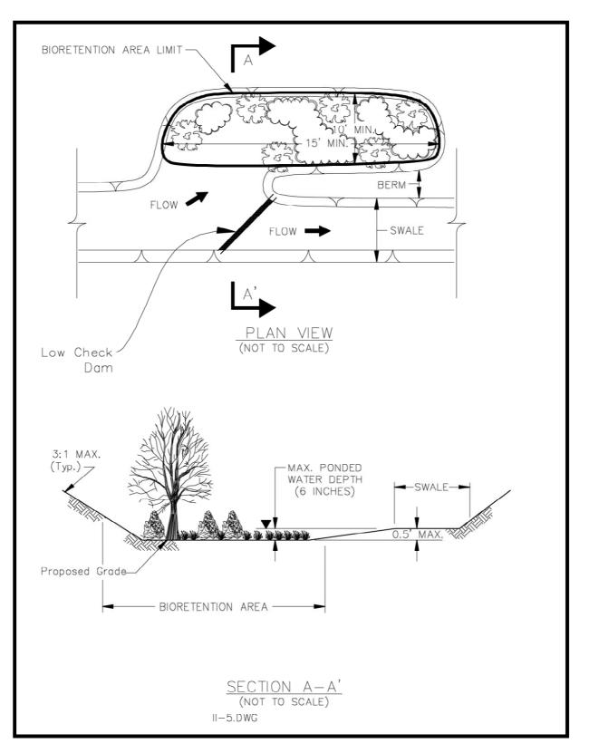
FIGURE 14.08-4 Bioretention Basin Adjacent to a Drainage Swale
