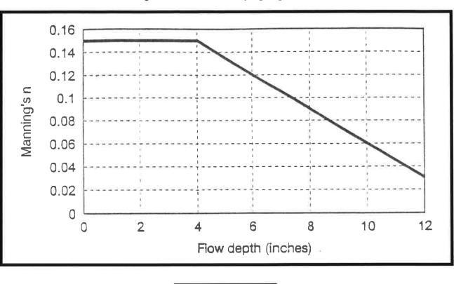
FIGURE 14.07-4 Manning's 'n' Values for Varying Depths of Flow
